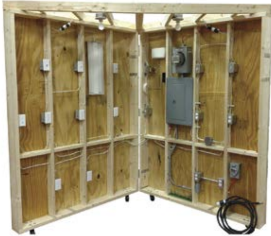
RESIDENTIAL WIRING DEMONSTRATOR
